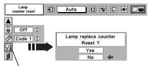
Move the pointer to Lamp counter reset and then press SELECT button. The message "Lamp replace counter reset?" is displayed.
